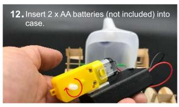
Use adhesive tape to stick motor to battery case First, ensure the motor is turning clockwise! (if not flip it over)
